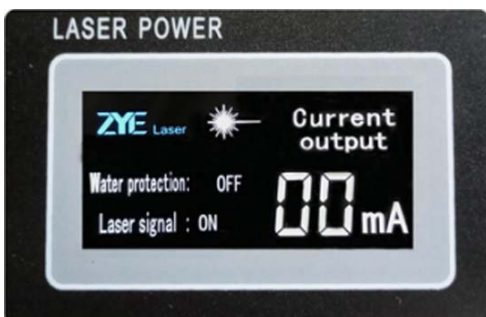
Display condition for no water protection
