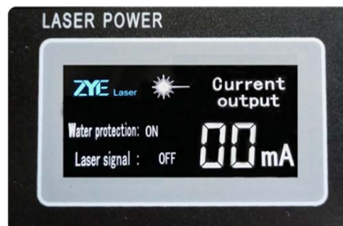
Display condition for no laser signal
