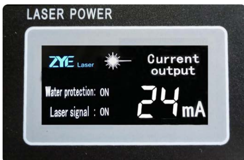
Display condition for normal working
