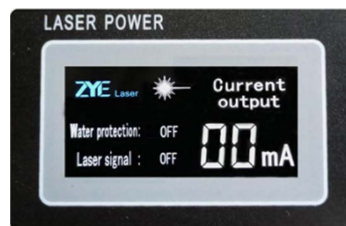
Display condition for neither water protection nor laser signal
