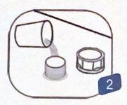
Open the injection port and add water. For best results, use deionized water.
