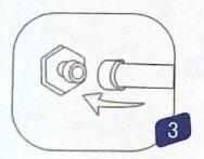
Connect the water inlet and outlet pipes to the system you wish to cool.
